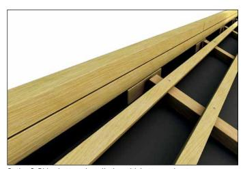
Option 2: Ridge batten - installation with batten understructure
