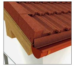
Adjust the Box Barges in a straight line and fix them using nails or fasteners. Note that the fasteners need to be near the bottom edge of the Box Barge to ensure that the bottom edge is firmly positioned against the barge board.
