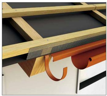
Option 2: Protection flashing going into the gutter
