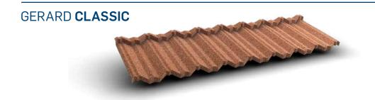
Length of Tile: 1320 mm Length of Cover: 1265 mm Width of Cover: 369 mm Tiles/m<sup>2</sup>: 2.14 Minimum Pitch: 12° (21%)
