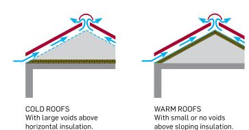
The harmful effects of condensation and ice damming can be avoided by ensuring that all the components of the roof are correctly installed. The tiles should be installed on a traditional batten structure. The roof should be designed as a ventilated system with an open-ended ventilation space. breathable underlay, thermal insulation and vapour membrane. It is recommended that a heat loss calculation is carried out according to local regulations.
