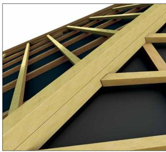
Option 2: Hip batten - installation with batten understructure
