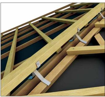
Option 1: Hip batten - installation with bracket
