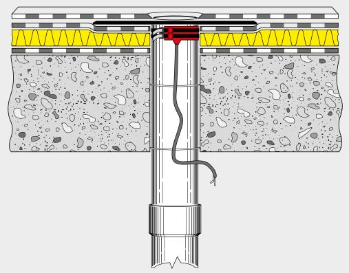
ITALPROFILI® **HEATING TAPE SYSTEM** is the perfect answer the overcoming the freezing problem of outlets and pipes of all types, whether fitted on new applications or as a retro fit product. Installation is quick and easy as the tapes need only to be positioned around the pipe and tightened in place using the fasteners.
